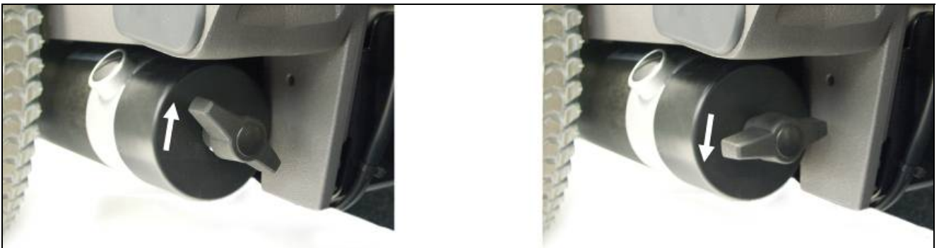
Figure 5.1: Links: free wheel switch in 'push' position; Right: 'drive' position
