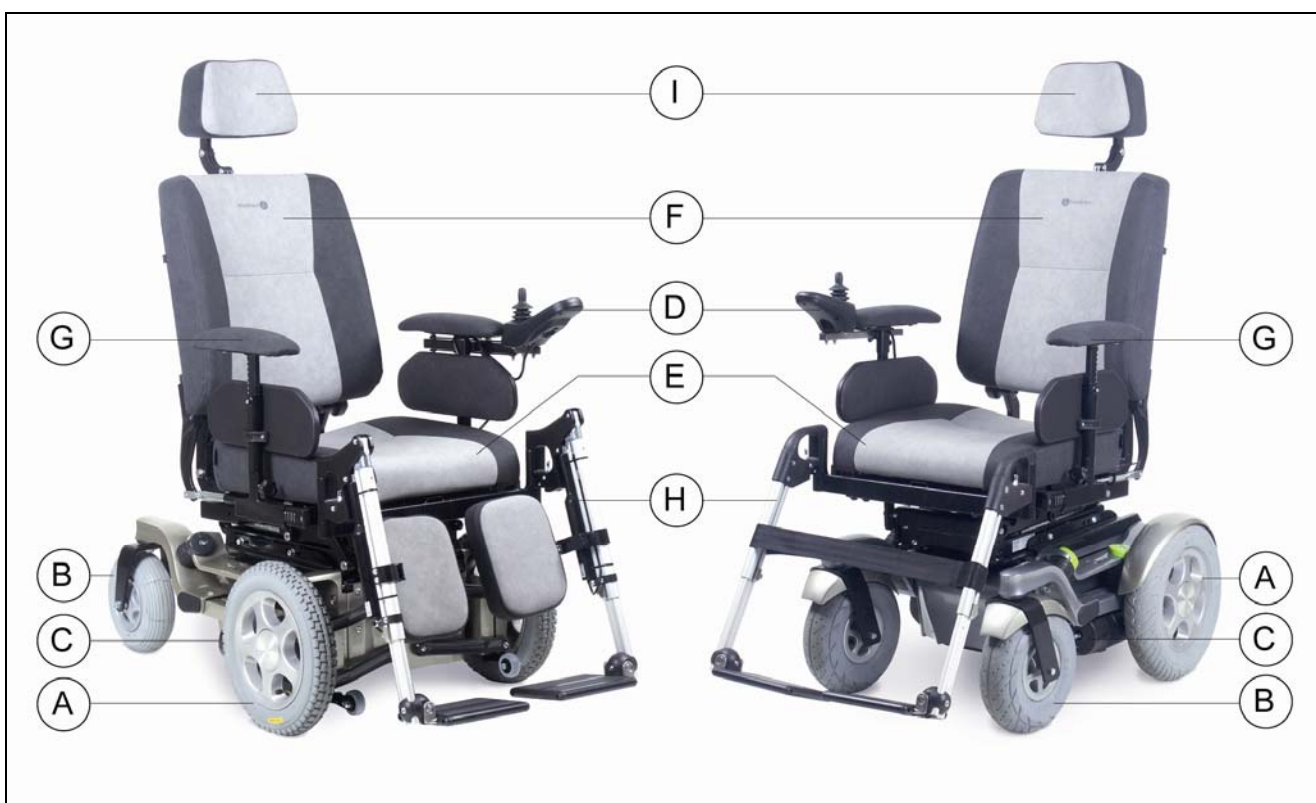
Figure 2.1: left front wheel driven (FWD), right rear wheel driven (RWD)
